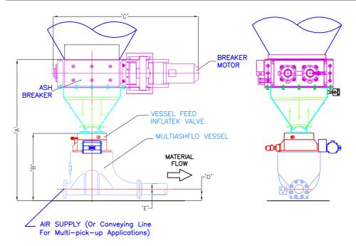
The **MultiAshflo and Ash Crusher Assembly** was developed for the special needs of hot bottom ash from a wide range of boiler stoker designs when the ash pit is not exposed to the radient heat of the combustion process. The assembly is designed for ash clinkers to 600mm in size and for their reduction in size to nominally 25mm. Also to handle clinkers at 650 °C.
