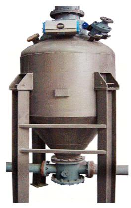
The **AshPump** is designed for efficient conveying of high rates of fly ash over long distances. It is normally located beneath utility Electro Static Precipitators (ESP) and Baghouses. Several **AshPumps** would be located on a single conveying pipeline to satisfy a high ash feed rate.
