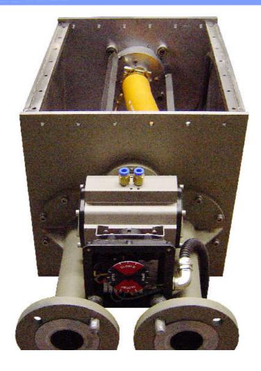
The **Type T Switch Valve** is used to form two branches in a conveying line handling cohesive or moist materials. It is self supporting in the conveying line and should be mounted vertically for best results. The valve action is self cleaning and does not leave any residual material between position changes.
