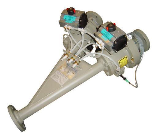
The **Type IV Switch Valve** is used to form two branches in a single conveying line handling large, lump material, and/or materials at high temperature. It is self supporting and may be mounted in the vertical, horizontal, or intermediate positions.
