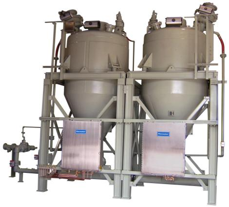
The **Macpump** is an arrangement of two pressure vessels working in an automatic and phased sequence to provide a continuous transfer of material with a high material pipeline loading for long conveying distances.
