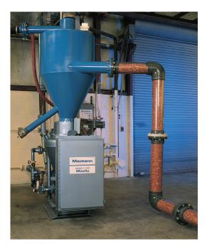
An example of a solid dense phase vacuum conveyor which may be applied to bulk container emptying requirements. Material velocity is extremely low without any particle duranticle. In this case shelled peanuts are conveyed from a bulk carrier without any degradation of the nut
